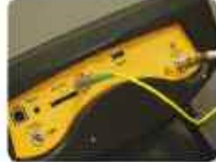
Combined with the triple light source OPS3L the H45 with optical receiver (optional) allows to check the response of an optical distribution network.
